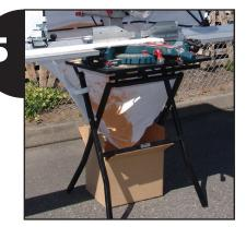
We recommend that you place a trash can or box under the ChopShop Saw Hood, which allows the dust and debris to collect in one spot.
