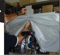
Unstrap the 3 Velcro hood wraps and let the saw hood fall into position.
