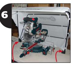
You can also mount the ChopShop Saw Hood to a table. Two mounting holes on each peacock tail will accept standard wood screws.
