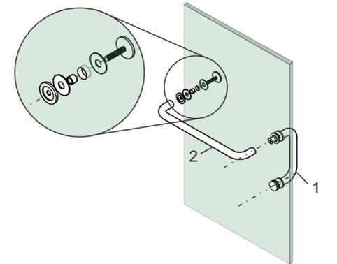
Install the set screws and tighten with the Allen key to finish the installation.
