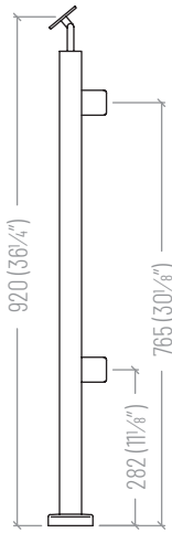
STAIR BOTTOM - Front
